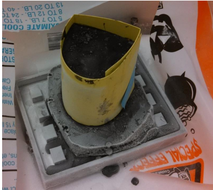
Figure 5 - Sample embedded in PVA, form still in place. The blade will slice from the right.
