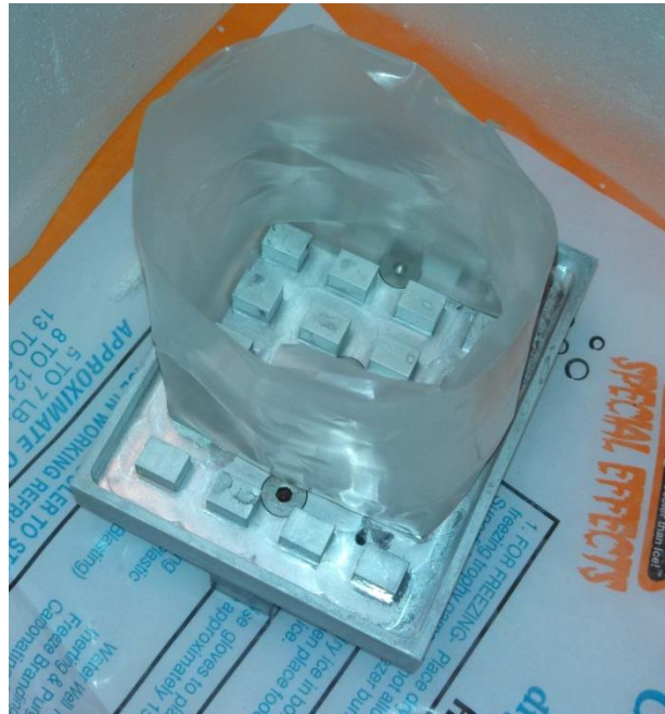
Figure 1 - example of a form for pouring the base
