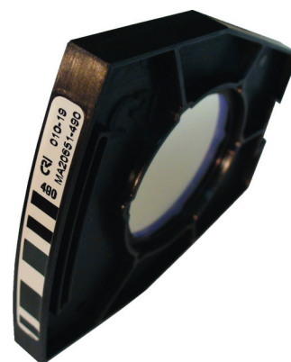
Figure 13. Emission Filter in its holder
